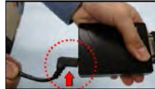
Do not apply excessive pressure to the USB cable and the terminal when connecting the main harness.
