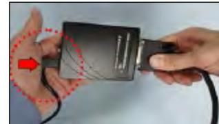
Connect the main harness gently in order to avoid excessive pressure to the USB plug.
